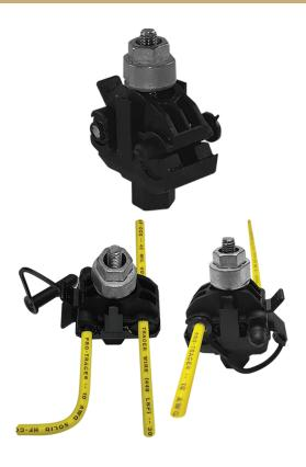
Tracer-Lock Connector is a direct bury, self-stripping, locking connector system used for corrosion proof and watertight connections to underground tracer wire systems. Our innovative and unique design allows the connector to be installed as an "in-line", "lateral" or "splice" connector without stripping the tracer wire.
