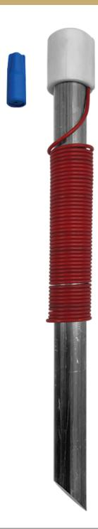
Ground Rods pull signal to avoid dispersion in multiple directions and complete the electrical circuit required to return signal back to the locate technician. (They) enable the signal transmission to travel much more fluidly, and enable the use of lower frequency to identify the line and prevent less signal bleed off (pinpoint accuracy) during the locate process.
